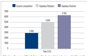
Filtration flow in a difficult thermoflashed red hybrid wine, with 2,2 mL/hL of Rapidase VinoFast, Contact time of 18 days at 18 °C (Canada).
